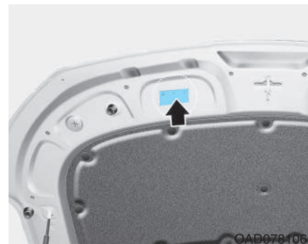
Air Conditioning refrigerant label
